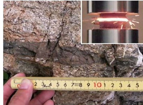
An example of natural pseudotachylyte (formed by frictional melting during an earthquake) and an experimentally reproduced melt layer.
