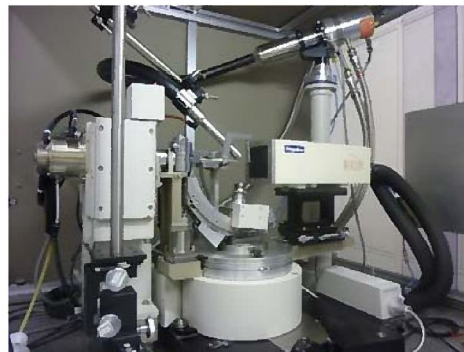
A four-circle X-ray diffractometer equipped with a CCD detector and sample-temperature controller.
